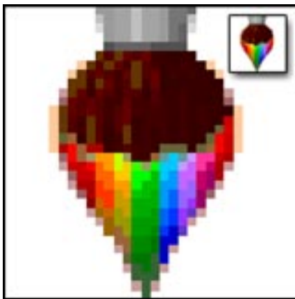
Raster Image: This is a simple representation of a raster image, a desktop icon which is presented at 32 by 32 pixels.
